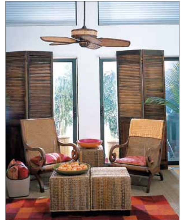
COOL DOWN: Mount ceiling fans at least 25-cm (10-inches) from the ceiling for adequate air circulation. COURTESY OF MONTE CARLO FANS
