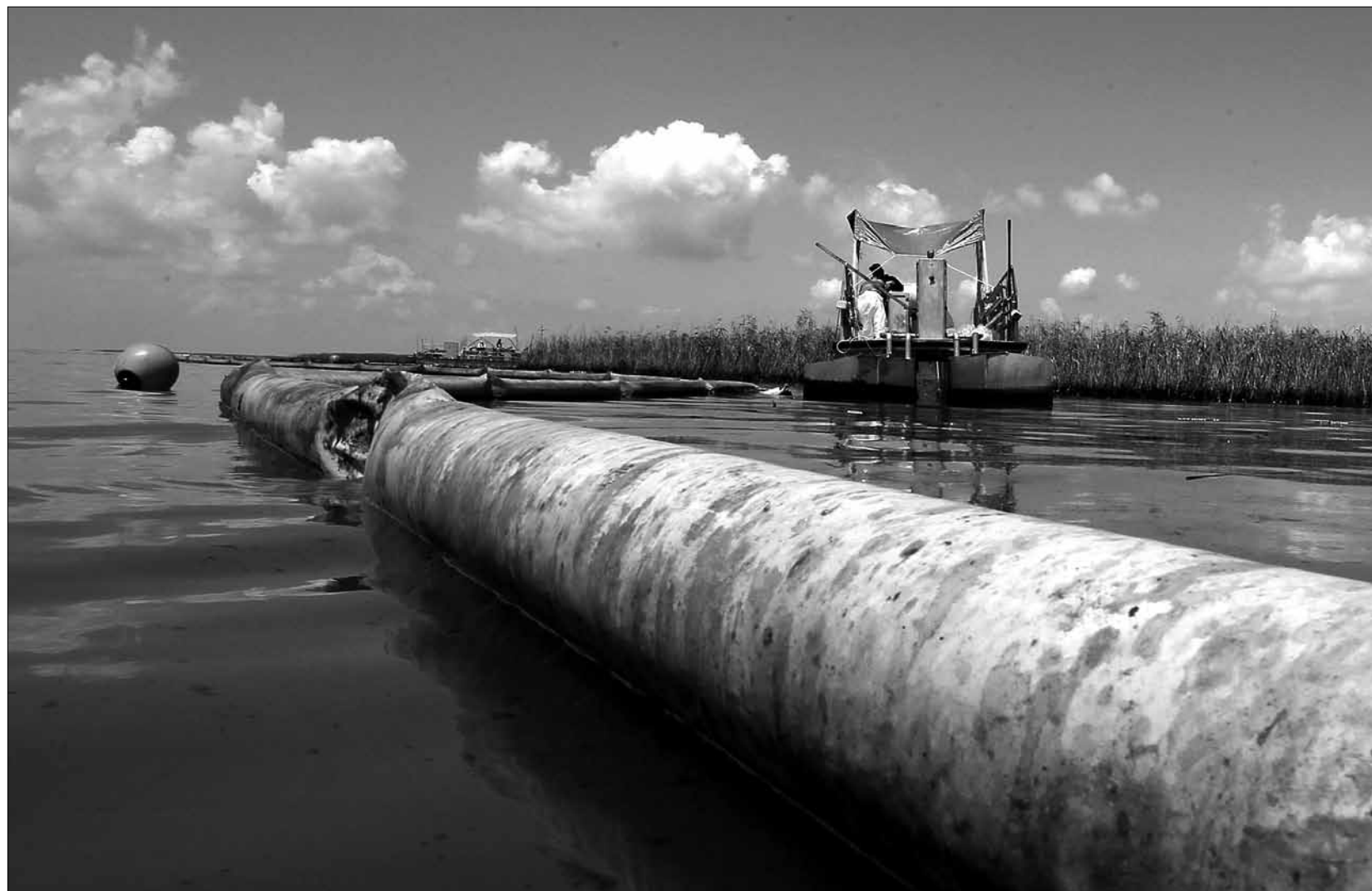
A boom floats in the water as contract workers from BP use skimmers to clean oil from a marsh on June 1. "Flotels" have been set up to provide housing for workers who are helping with the clean up. WIN MCNAMEE/GETTY IMAGES
